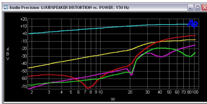
Figure 313. Fundamental (top curve), 2nd harmonic, 3rd harmonic, 4th harmonic, and 5th harmonic amplitudes of a loudspeaker as a function of power.
