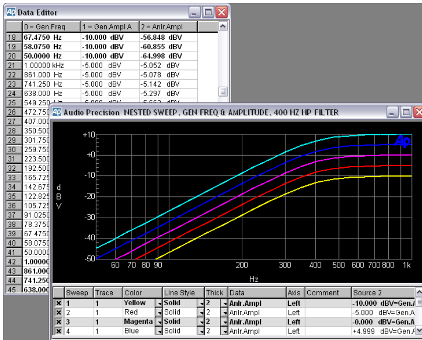
Figure 336. Graph Legend and Data Editor, showing the linked relationship of the typefaces used in the two displays, for a nested sweep.
