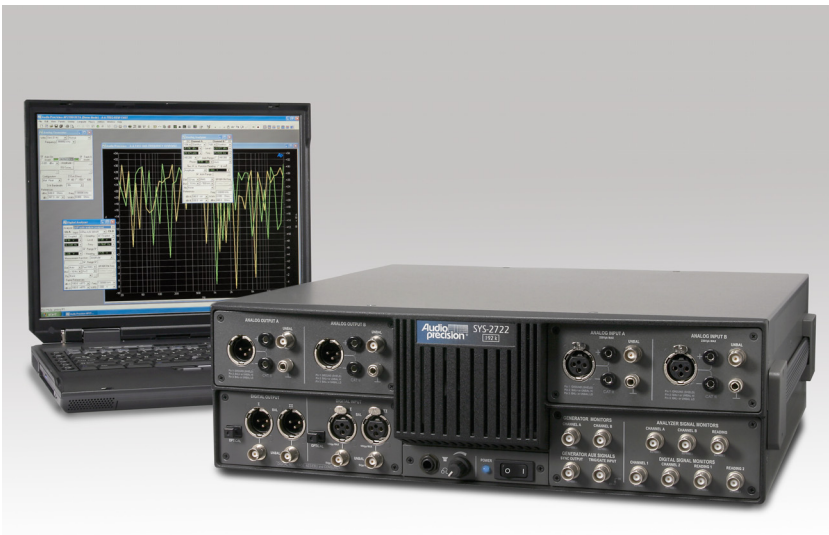
Figure 1. An Audio Precision 2700 series audio test and measurement instrument (SYS-2722 shown).
